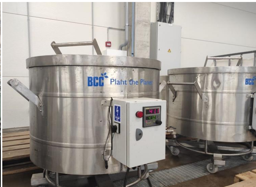
Oak thermotherapy line processing up to 50 tons of depth per season
